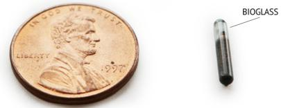
It is important to clarify a microchip is NOT a GPS or tracking device because it has no power source! Instead, a microchip contains a small antenna that can only be read by a microchip scanner used by veterinarians, shelters, and animal control. When the scanner passes over the microchip, it reads the microchip ID number. It is not exactly the same, but similar to scanning a barcoded item at the grocery store.
